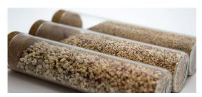
To reach a spot-free drying and a light polishing the parts often pass through a dryer filled with maize corn cob after the treatment. Maize corn cob is a pure natural product. It is produced by crushing, sieving and dedusting of maize husks (ginned maize corn cobs). The granulate is available in different sizes.
