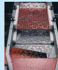
Separation on two levels – parts on the upper and undersize media on the lower level.
